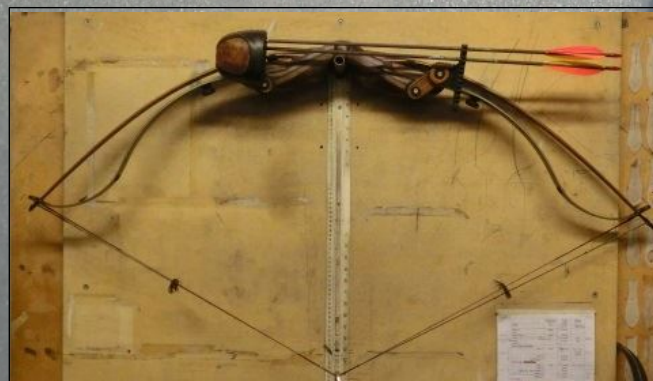
Covert Hunter and Hawk Hunter longbow similar string angles at full draw 28"
